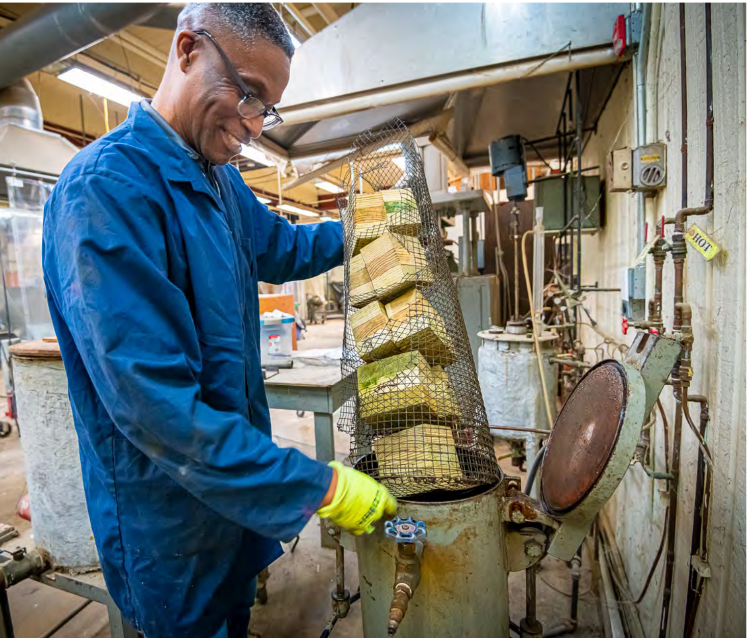
Franklin Quin places CLT samples in a dryer. (Photo by David Ammon)
