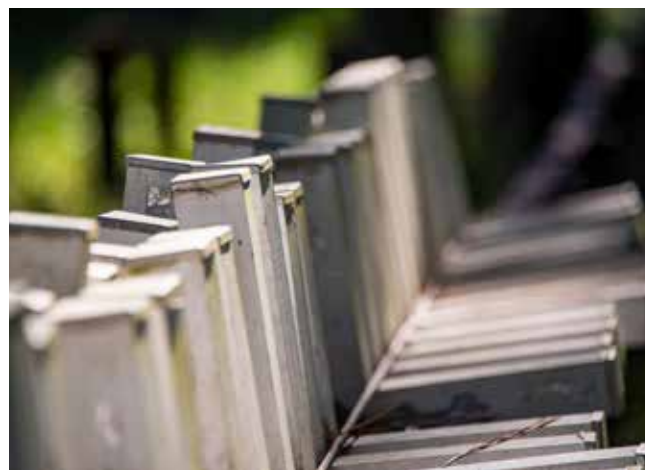
Long-term wood preservation test in an outdoor laboratory. (Photo by David Ammon)
