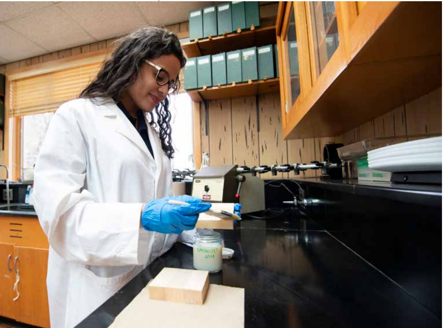
Dr. Gabrielly Dos Santos Bobadilha applies a coating to cross-laminated timber. (Photo by David Ammon)
