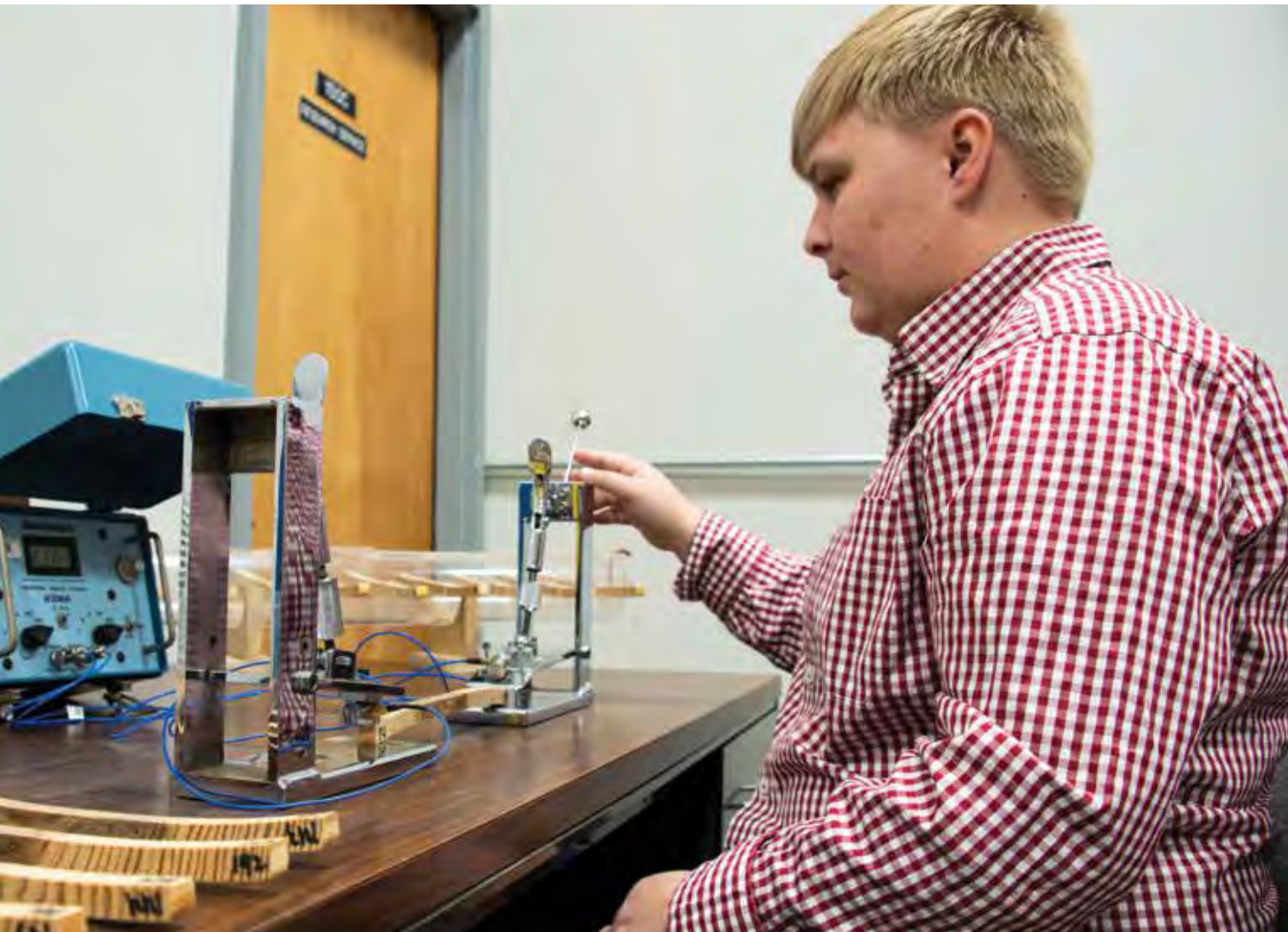
Brianna Duquette tests the tension of wood infected with brown rot to determine strength (Photo by Dominique Belcher)
