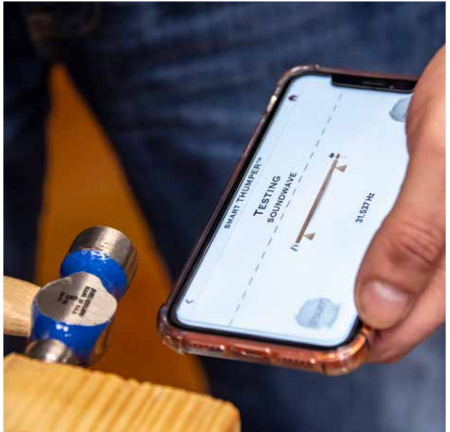
The Smart Thumper app uses sound or vibration to evaluate lumber. (Photo by David Ammon)
